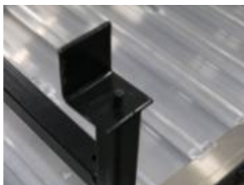
4. Lift Bracket and Pull Steps towards Trailer until Pin is Inserted into Lock Hole on Step Frame.
