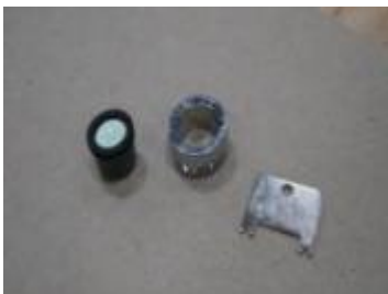
Dis Assembled Aerator.
