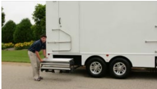
2. Pull Steps Out and Lock in Place With Spring Loaded Pins
