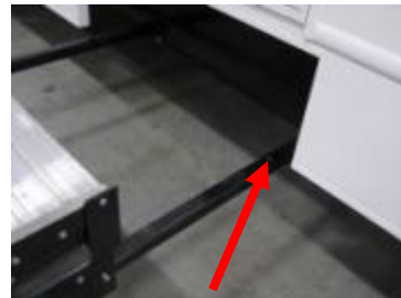
4. Lift Bracket and Pull Steps towards Trailer until Pin is Inserted into Lock Hole on Step Frame.
