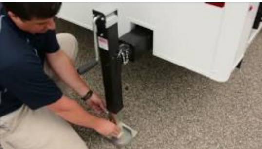
4. Adjust Height and Insert Pin.
