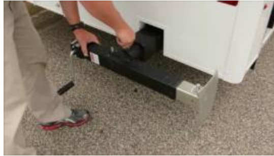
1. Remove Keeper Pin then rotate 90 degrees
