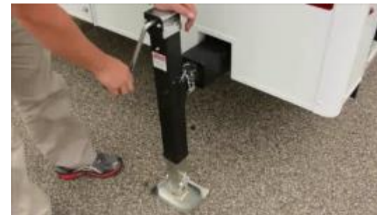
5. Once in contact with the ground rotate three to five times.
