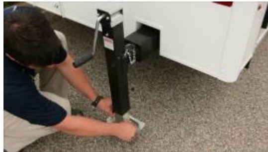
3. Remove Quick Adjust Pin.
