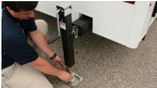
4. Adjust Height and Insert Pin.
