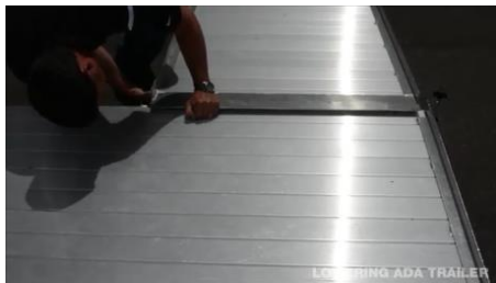
Secure Ramp by Aligning Pins in Holes to Platform
