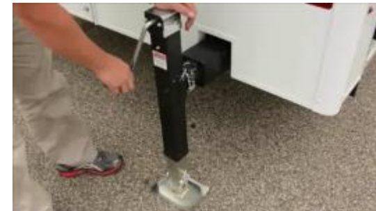
5. Once in contact with the ground rotate three to five times.
