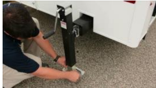
3. Remove Quick Adjust Pin.
